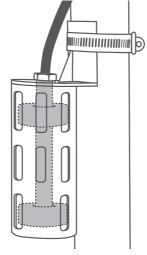
second switch. As the pump evacuates the water from the pit, the floats will drop. The pump will run for an additional 10 seconds to extend the cycle after the float returns to its original position.
