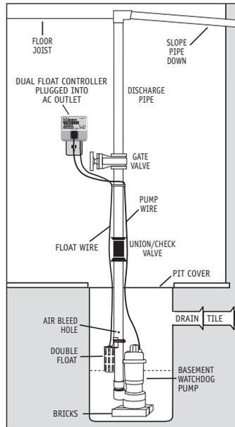
7. Install a gate valve or ball valve if required by any codes.
