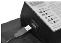
*Note: When using the data connection, no other cable is necessary; this cable will also power the WiFi module. However, we recommend connecting the mini USB cable and USB charger in order to provide an additional power source to the WiFi module.*
