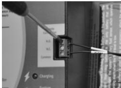
2. On the same end of the remote terminal cable, attach the cable end labeled 'COM' to the Common port labeled 'COM' on the back or side of the backup system control box. Turn the screw clockwise to secure the wire.
