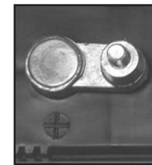
POSITIVE POST HAS LARGER DIAMETER
