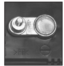
NEGATIVE POST HAS SMALLER DIAMETER
