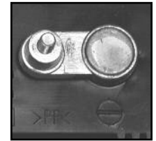
NEGATIVE POST HAS SMALLER DIAMETER
