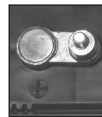
POSITIVE POST HAS LARGER DIAMETER
