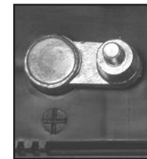
POSITIVE POST HAS LARGER DIAMETER
