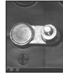
POSITIVE POST HAS LARGER DIAMETER
