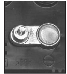
NEGATIVE POST HAS SMALLER DIAMETER
