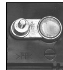
NEGATIVE POST HAS SMALLER DIAMETER
