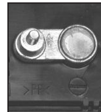
NEGATIVE POST HAS SMALLER DIAMETER
