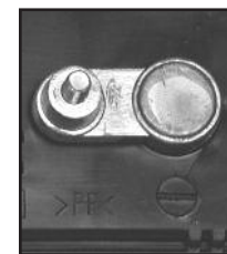
NEGATIVE POST HAS SMALLER DIAMETER
