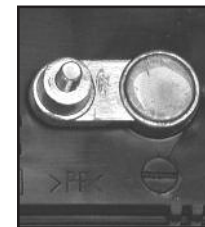
NEGATIVE POST HAS SMALLER DIAMETER
