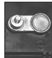
NEGATIVE POST HAS SMALLER DIAMETER
