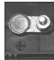
POSITIVE POST HAS LARGER DIAMETER
