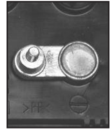
NEGATIVE POST HAS SMALLER DIAMETER
