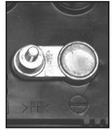
NEGATIVE POST HAS SMALLER DIAMETER
