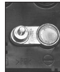
NEGATIVE POST HAS SMALLER DIAMETER
