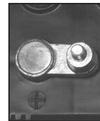
POSITIVE POST HAS LARGER DIAMETER
