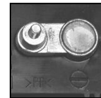
NEGATIVE POST HAS SMALLER DIAMETER
