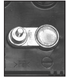
NEGATIVE POST HAS SMALLER DIAMETER
